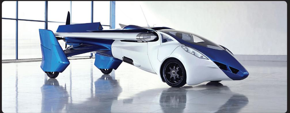
idea was finally brought to life by Štefan Klein, who began working on the invention in 1989. The AeroMobil 3.0 is essentially a two-person sports car with wings that tuck in while on the road and fold out for flight.
